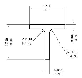
(AS SHOWN) WALL THICKNESS EXCEPT AS SHOWN DATE REV DESCRIPTION BY 03/21/23 REMOVED ALLOY NDZAL 350.857 мм.<sup>2</sup> 0.544 IN.<sup>2</sup> EST.AREA EST.AREA 0.955 0.642 EST.WT. LBS/FT. EST.WT. KG/M. 5.839 148.301 EST.PER. MM. EST.PER. OUT PER. MM. OUT PER. 1.880 C.C.D. 47.753 C.C.D. FACTOR 9 **FINISH** M/F ALLOY & TEMP. DWN BY C.P.SCALE 1:1 DATE 01/15/2001 CKD BY
